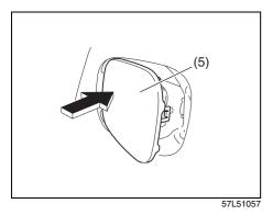
From the outside, push the part indicated by the arrow of the fuel filler door (5) (see the illustration). The door will open slightly.
